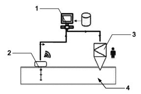
This autonomous aquaculture fish feeding system comprises an autonomous vessel (2) having multiple temperature and salinity sensors; an electronic data processor (1) configured to use sensor collected information to calculate a fish weight prediction model for each prediction model segment.
